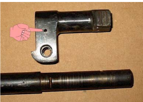
Location of the front sight assembly, rear retaining pin.
