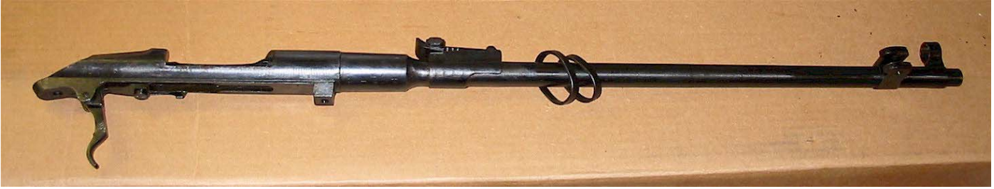
The simplicity of the Mosin Nagant M44 action is illustrated above.
